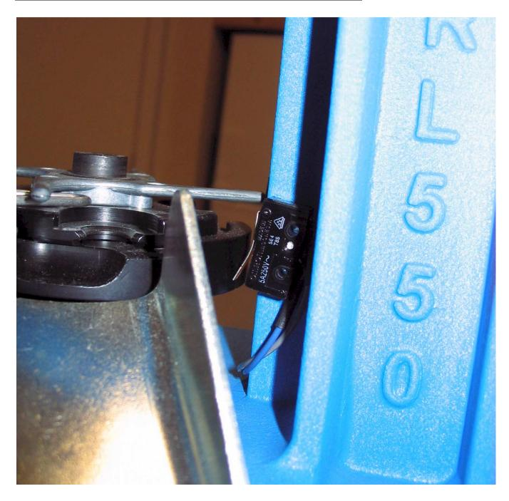
The best place to sense the handle up on the Dillon 550 is on the right side of the rear column. Note that this shell plate is at rest and that the end of the lever is near the bottom of the shell plate. This allows the shell plate to drop slightly further when priming is occurring and still the end of the lever will be activate and will not reach the top of the shell plate.
