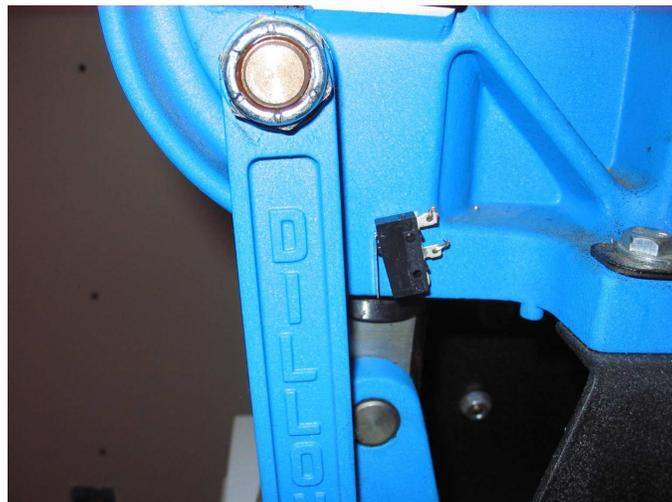
**Press Handle Down Sensor:** The best place to sense the handle down on the Dillon 650 is on the right side of the press where the handle linkage travels.
