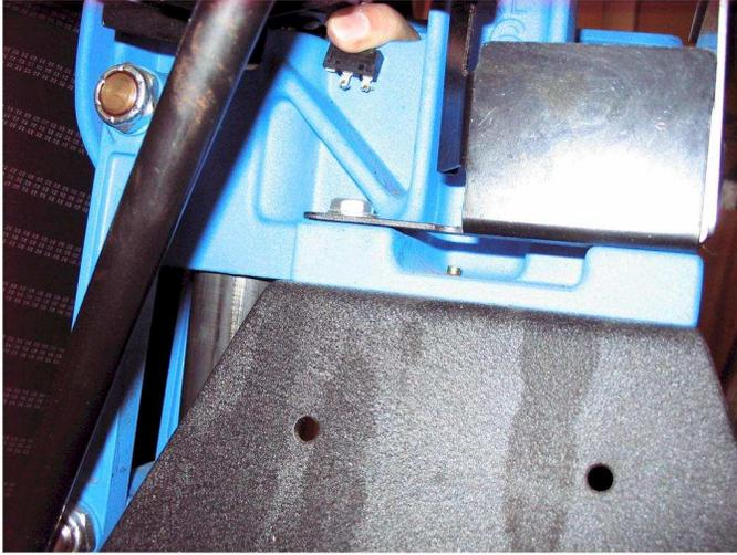
**Press Priming Sensor:** The best place to sense the handle up on the Dillon 650 is on the right back side of the press where there is a nice flat surface to mount the sensor. It should be mounted so that the lever is pointing towards the user. There is something that comes down with the shellplate that will hit it in this location.
