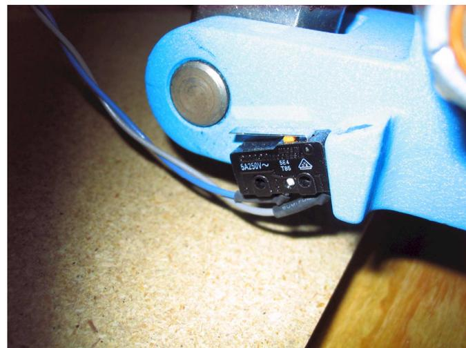
**Press Handle Down Sensor:** The best place to sense the handle down on the Dillon 550 is on the handle linkage itself.
