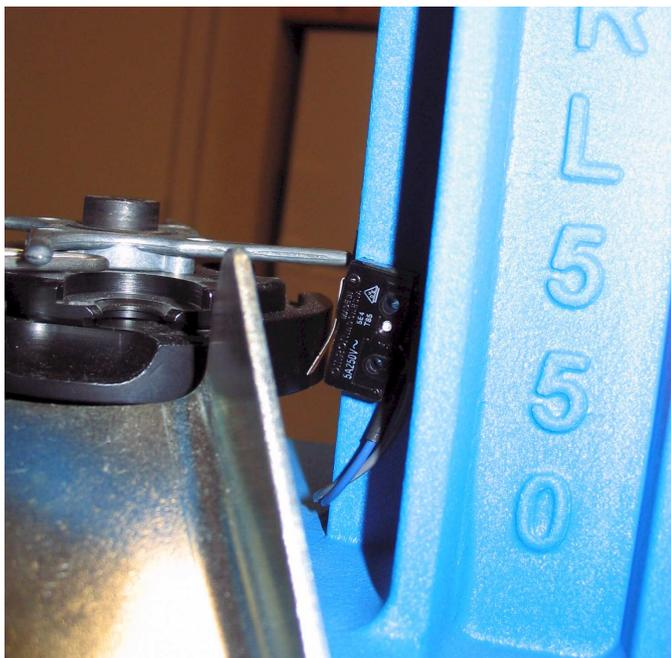
**Press Priming Sensor:** The best place to sense priming on the Dillon 550 is on the right side of the rear column.
