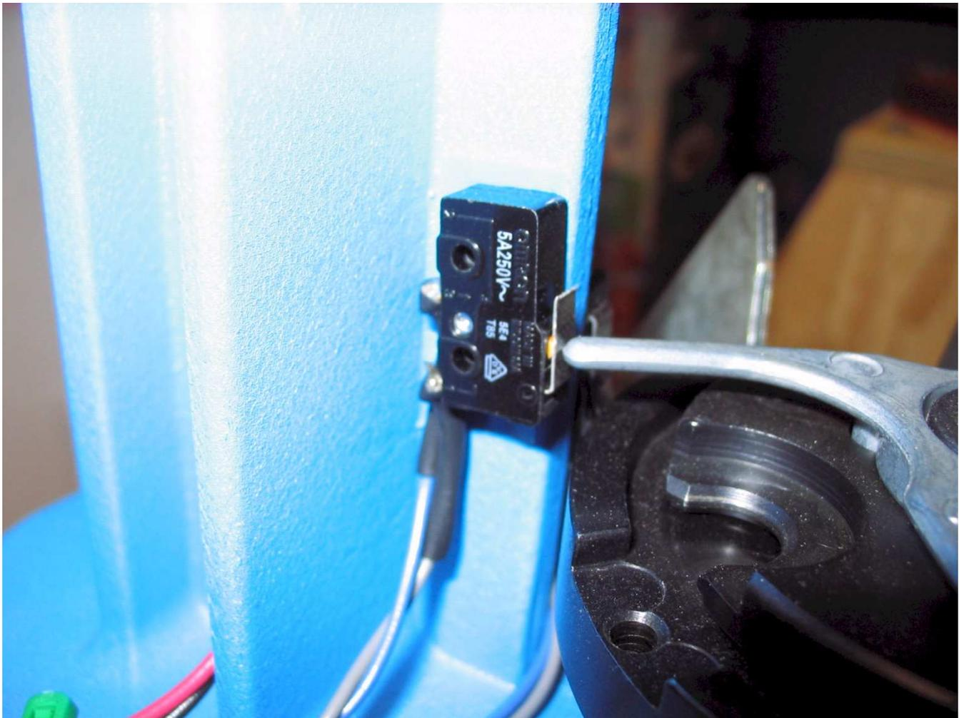
This is the switch that detects the star movement when the shellplate is rotated. It should be mounted on the left of the column so that the lever points up so that the star hits it as it goes by. Put the switch in place when the star is contacting it (like in the picture above). A very slight amount of counter clockwise skew helps. Just make sure that when the shellplate comes back down it is no where near hitting the end of the lever.
