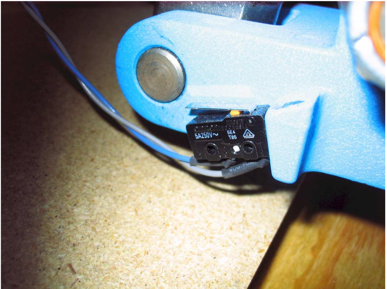
The handle down sensor senses when the handle is down and on the Dillon 550, the best place to sense this is on the handle linkage itself. Note that when the handle is fully down, there is no pressure on the switch itself, just that the switch lever is activated.
